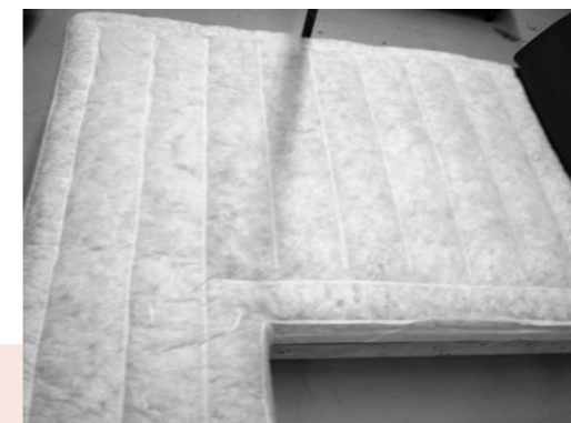
Very loose, chamber cushion without cover
